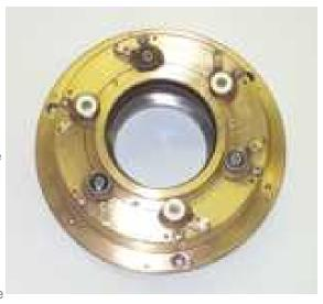
tube ends; variation in the concentricity between the tube and rotating chamber gives rise to ultrasonic incident angle variation with resulting sensitivity variations and the repeatability statistics of the overall system deteriorates.
